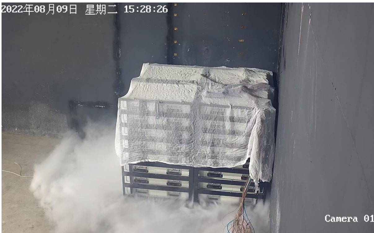
Figure 13. Photo 02 of initiating BESS unit and target BESS units during test.
